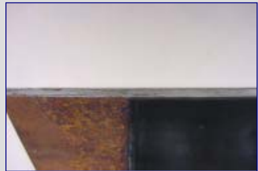
Test sample slice no delamination
