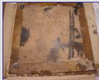
Test sample after five months in a baghouse
